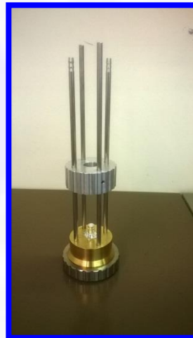
The Sonemat HWS2235-WCT EMAT is able to operate on samples at temperatures of up to 800c with active water cooling.
